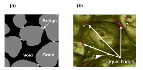
FIG. 1. Illustration of isolated bridges at low levels of saturation. (a) Micro-x-ray computer tomography (MicroXCT) image, typical from our experiments. (b) 3D image reconstruction of MicroXCT data. The liquid within the grain roughness is invisible to MicroXCT, since resolution is limited to a few micrometres.
