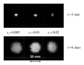
FIG. 18. Spreading of TEHP liquid drops  $(V_D = 6 \,\mathrm{mm}^3)$  in pre-wetted sands with different background saturations levels  $s_r = 0.5, 1$  and 2%. UV fluorescence wet spot areas taken at  $t = 3 \,\mathrm{min}$  and at  $t = 6 \,\mathrm{days}$  after the deposition of the drops on the sand bed.
