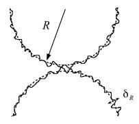
FIG. 2. The contact zone between two rough spherical particles
