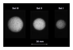
FIG. 4. UV fluorescence images of wet areas taken after  $\approx$  45000 min of spreading from above the sand bed prepared using  $R \approx 0.26$  mm sand. From left to right the image is for the sets III, II and I, as in Table I.
