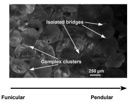
FIG. 3. An UV fluorescence image of the liquid (TEHP) distribution in sands in the transition from the pendular to the funicular regimes of wetting, at s > 10%.
