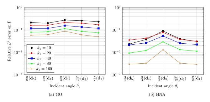
Figure 9: Accuracy of GO and HNA approximations to  $u_1$  on  $\Gamma$  plotted against incident angle  $\theta_i$  for the incident directions  $\mathbf{d}_1, \ldots, \mathbf{d}_5$  of Figure 7(a), for  $\alpha = 1$  and  $\mu = 1.5 + 0.003125i$ .
