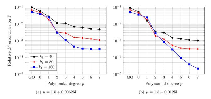
Figure 6: Numerical best approximation errors for the configuration in Figure 1 at two different refractive indices (left panel - lower absorption, right panel - higher absorption), as a function of polynomial degree p. Other approximation space parameters ( $C_{np}$  etc.) are as specified in §4. For reference the GO error is also shown.
