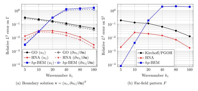
Figure 8: Scattering by an equilateral triangle with  $\mathbf{d}^i = \mathbf{d}_1$ ,  $\alpha = 1$  and  $\mu = 1.5 + 0.003125$ i. Errors in boundary solution and far-field pattern for GO (Kirchoff/PGOH in the far field), our HNA BEM (with fixed N = 416) and a conventional hp-BEM (with fixed N = 456).
