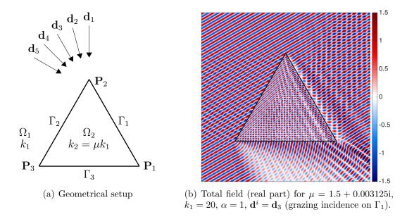
Figure 7: Scattering by an equilateral triangle.
