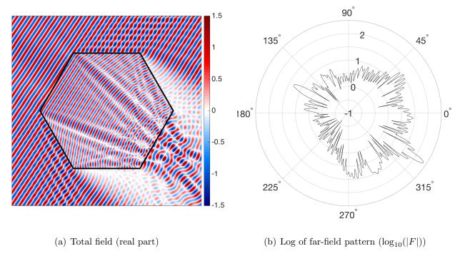
Figure 15: Scattering by a regular hexagon with  $k_1 = 10$ ,  $\mu = 1.39 + 0.00667$ i,  $\alpha = 1$ , and incident angle  $\theta_i = \tan^{-1}(2/3)$ .
