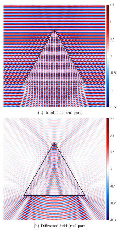
Figure 1: Scattering by an equilateral triangle of side length  $2\pi$  and refractive index  $\mu = 1.5 + 0.003125i$ , computed using our HNA BEM. Here  $k_1 = 20$ ,  $\alpha = 1$ , and the incident wave arrives from above, corresponding to  $\mathbf{d}^i = \mathbf{d}_1$  in the geometrical setup described in Figure 7(a).
