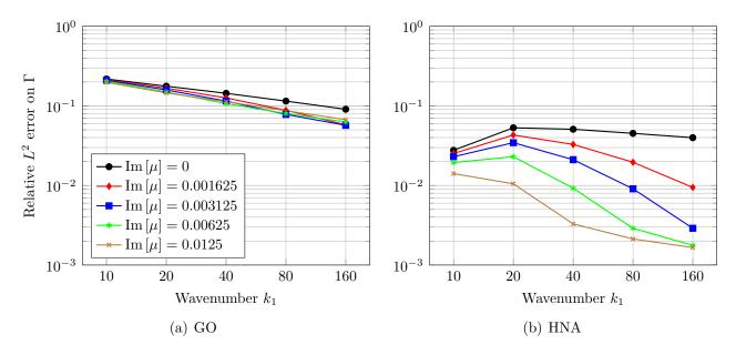
Figure 14: Accuracy of GO and HNA approximations to  $u_1$  on  $\Gamma$  for the triangle with  $\alpha = 1$  and  $\mathbf{d}^i = \mathbf{d}_5$  ( $\theta_i = \pi/6$ ), with Re  $[\mu] = 1.5$  and Im  $[\mu]$  varying between 0 and 0.0125.
