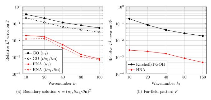
Figure 16: Accuracy of GO and HNA for scattering by a regular hexagon with  $\mu = 1.39 + 0.00667$ i,  $\alpha = 1$ , and incident angle  $\theta_i = \tan^{-1}(2/3)$ .
