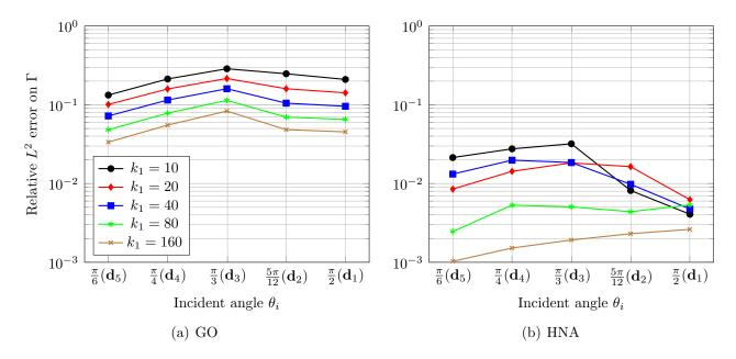
Figure 10: Accuracy of GO and HNA approximations to  $u_1$  on  $\Gamma$  plotted against incident angle  $\theta_i$  for the incident directions  $\mathbf{d}_1, \ldots, \mathbf{d}_5$  of Figure 7(a), for  $\alpha = 1$  and  $\mu = 0.66 + 0.003125i$ .
