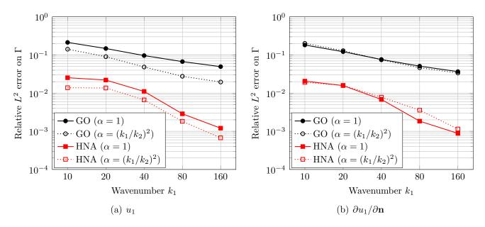
Figure 13: Accuracy of GO and HNA approximations to  $u_1$  and  $\partial u_1/\partial \mathbf{n}$  on  $\Gamma$  for the triangle with  $\alpha = 1$  and  $\alpha = (k_1/k_2)^2$ , with  $\mu = 1.5 + 0.00625$ i and  $\mathbf{d}^i = \mathbf{d}_1$  ( $\theta_i = \pi/2$ ).
