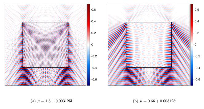
Figure 12: Real part of the diffracted field for a square with different real part of the refractive index. The incident wave is directed from above.
