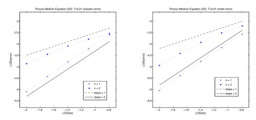
Figure 17: Accuracy of the approximate solutions to the two-dimensional porous medium equation (n = 1 and n = 2) on a sequence of meshes at T = 0.01 obtained using the scale-invariant arclength monitor integral: solution error (left) and mesh error (right) both in the  $L_1$  norm.
