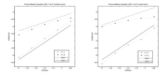
Figure 3: Accuracy of the approximate solutions to the two-dimensional porous medium equation (n = 1 and n = 2) on a sequence of meshes at T = 0.01 obtained using the standard scheme but with a non-zero vorticity added to the mesh velocity field: solution error (left) and mesh error (right) both in the  $L_1$  norm.
