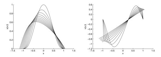
Figure 12: Evolution of the solution (left) and mesh velocity (right) for the one-dimensional Richards equation, reproduced from [131].
