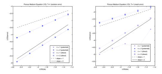
Figure 7: Accuracy of the approximate solutions to the one-dimensional porous medium equation (n = 1 and n = 2) on a sequence of meshes at T = 1.0 obtained by recovering the velocity directly and via a potential: solution error (left) and mesh error (right) both in the  $L_1$  norm.
