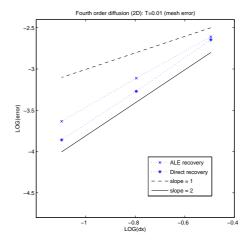
Figure 8: Accuracy of the approximate solutions to the two-dimensional fourth order nonlinear diffusion equation (n = 1) on a sequence of meshes at T = 0.01 obtained using the standard scheme: solution error (left) and mesh error (right) both in the  $L_1$  norm.
