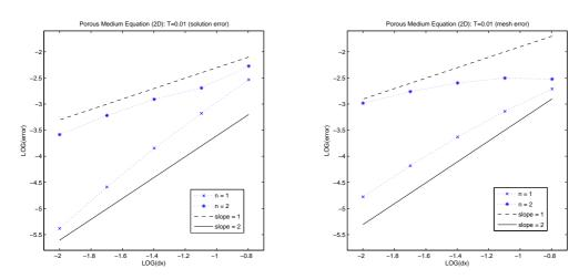
Figure 5: Accuracy of the approximate solutions to the two-dimensional porous medium equation (n = 1 and n = 2) on a sequence of meshes at T = 0.01 obtained with upwinded velocity recovery: solution error (left) and mesh error (right) both in the  $L_1$  norm.
