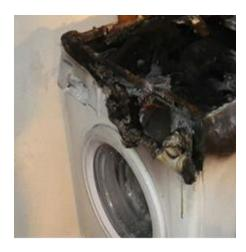
The main reason for a tumble dryer to catch fire is a clogged up lint filter. Depending on the frequency of use of the dryer the lint filter may need cleaning on a daily basis. Also, make sure that the vent pipe (if fitted — some condenser dryers do not need one) is not blocked or kinked in any way. Finally do not put any materials that have
