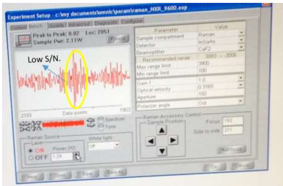
Figure 5. Example of a bad sample FT Raman interferogram, whose S/N is very low.
