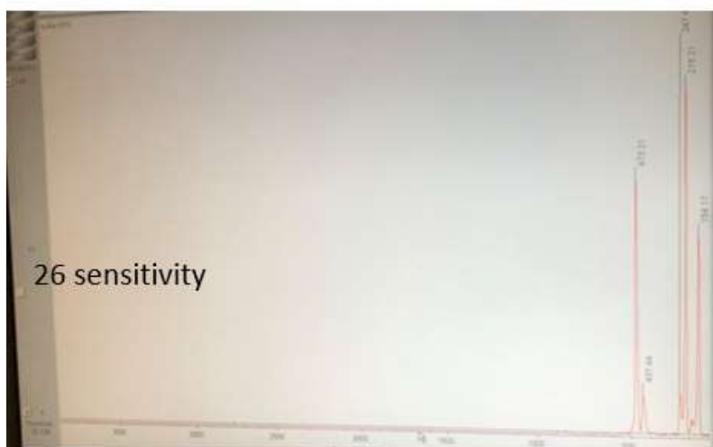
Figure 16. Example of how sensitivity value affect the labelling process in a S2 spectrum. Same threshold (at the bottom of the spectrum) in both cases.
